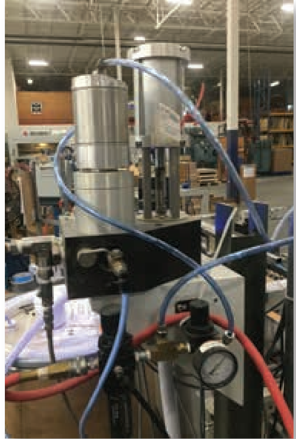
PFRM-5 Option offers one-piece glue source for easy installation and cost effective price. Includes piston pump, in-line filter, pressure-balancing regulator and output manifold
